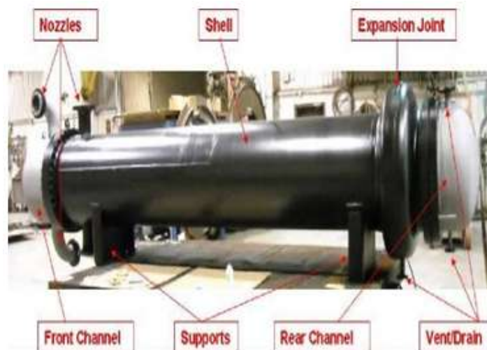
fig :- Construction of STHE
